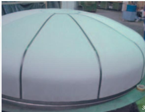
FRP is a composite material made of resin and glass. The liquid reaction resins used are unsaturated polyester resins and vinyl ester resins. The glass used for reinforcement is integrated in the form of roving, matting and meshing. The join of resin and glass to create a load-bearing structure is termed laminate.
