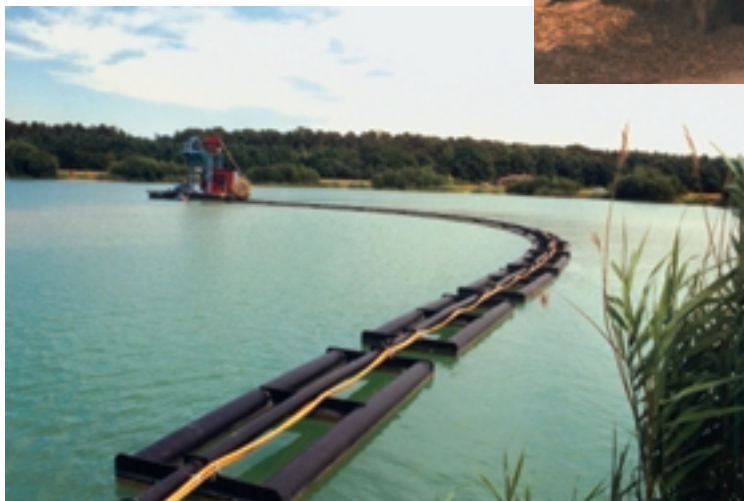
Floating dredger with suction pipe for removing fine sand and sludge. The floating dredger is positioned with the aid of an anchor boom.
