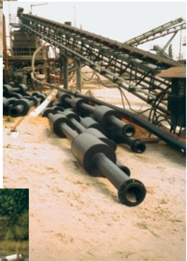
Low-cost solution with firmly integrated floats. The welded design minimises the cost of materials, but the floats can no longer be taken apart when the pipeline becomes worn.
