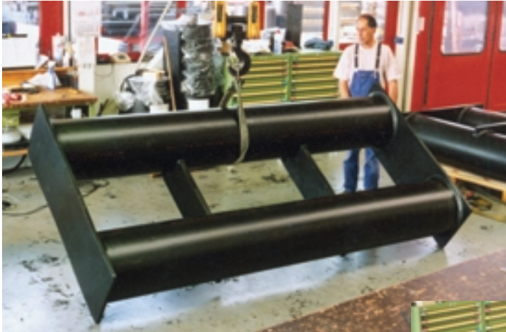
Factory production of the basic structure consisting of welded plates and pipes made of PE. The lower specific weight of polyethylene with a material density of 0.95 g/cm 3 facilitates handling of the individual elements when they are finished.
