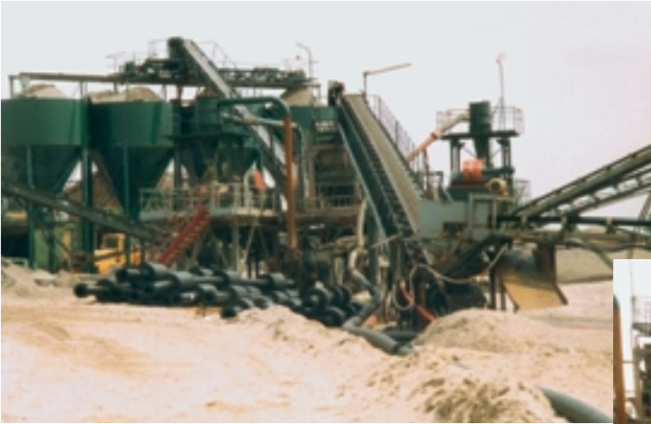
Sand and gravel classification plant with supply silos. It also serves as a storage depot for the individual elements when they are delivered.
