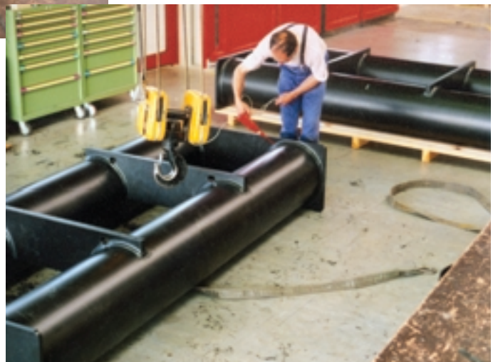
Final quality control with a continuous welding seam inspection by spark induction testing in accordance with DVS (German Association of Welding) guarantees a high level of safety.
