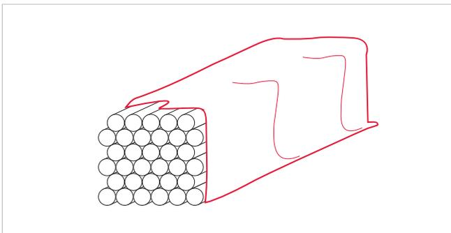
On-site storage in wooden frame under a light-coloured plastic sheet.
