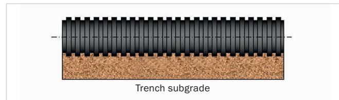
More elaborate configuration of trench subgrade for profiled pipes
