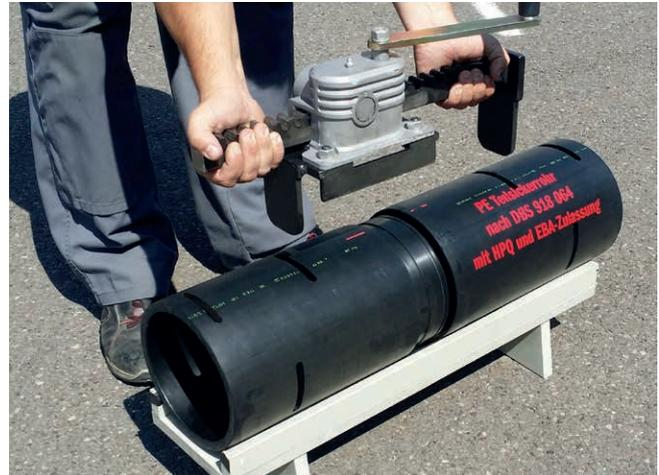
Fitting the manual insertion tool
